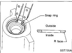
2. Install a new snap ring into gear housing.
