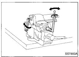
d. Measure turning torque at straight-ahead position.
