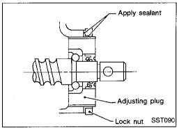
4. Apply suitable sealant to inner surface of lock nut.
