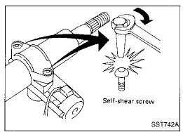
Install self-shear type screws, then tighten until heads break off
