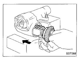
2. Place worm gear assembly together with worm gear bearing into gear housing.
