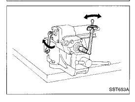
d. Measure turning torque at straight-ahead position.
