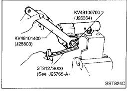
3. Adjust worm gear bearing preload using Tools.
