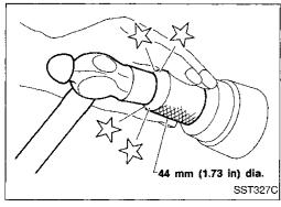
9. Install new oil seal into gear housing with suitable tool.
