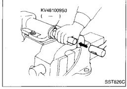
1. Press new oil seal and then install back-up ring with Tool.
